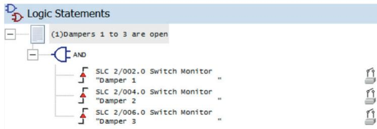
In this example, fan 1 is interlocked with dampers 1, 2 and 3. The fan will not attempt to run until feedback is received that all three dampers are open. The fire alarm control panel will only instruct the fan to start once the interlock logic is satisfied.
