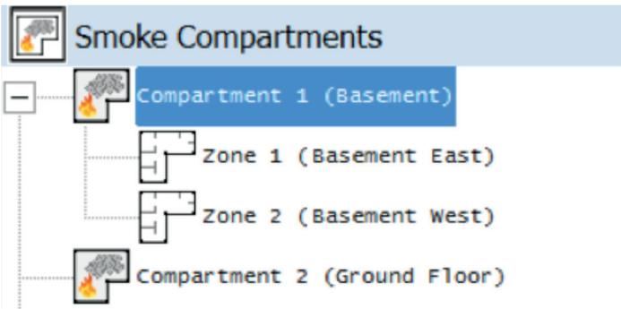
In the above example, the default setting means any alarm from a detector in zones 1 or 2 will initiate compartment 1 smoke control.
